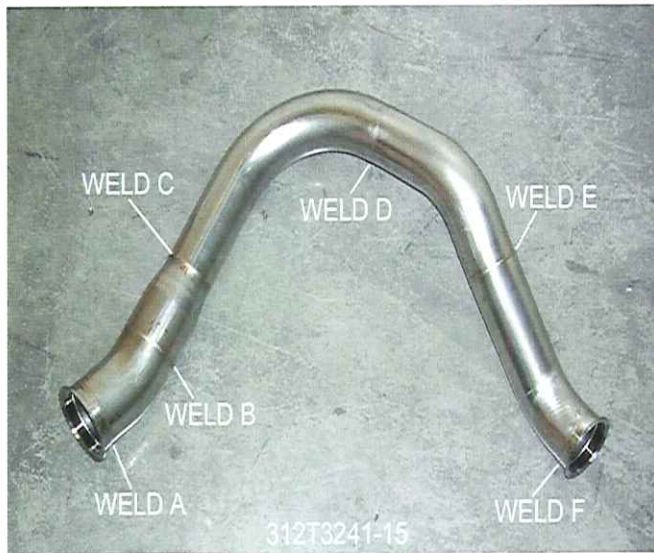
Inconel Ducting: Class A welds (100% inspection required) Controlling Specification BAC5975. Single-wall exposure setup.
